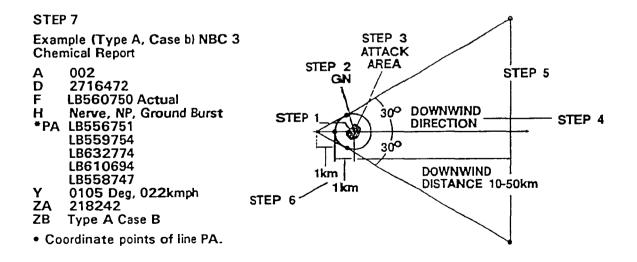
Figure 3-14. Plot for downwind hazard, Type A, Case b.
